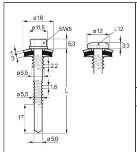
Fastener: Carbon steel with anticorrosion coating
