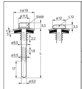
Fastener: Carbon steel with anticorrosion coating
