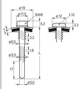
Fastener: Carbon steel with anticorrosion coating
