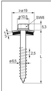
Fastener: Stainless steel A2 or A4 - EN ISO 3506 Washer: Stainless steel A2 or A4 - EN ISO 3506
