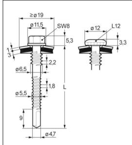
Fastener: Carbon steel with anticorrosion coating
