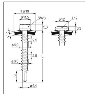
Fastener: Carbon steel with anticorrosion coating
