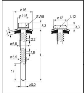
Fastener: Carbon steel with anticorrosion coating
