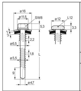
Fastener: Carbon steel with anticorrosion coating
