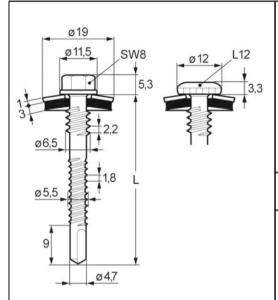
Fastener: Carbon steel with anticorrosion coating
