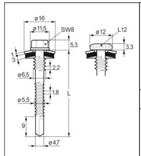
Fastener: Carbon steel with anticorrosion coating
