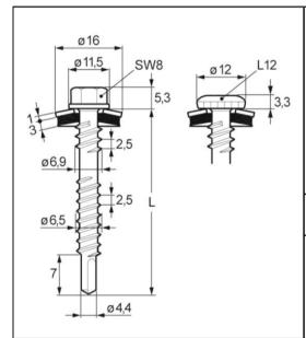
Fastener: Carbon steel with anticorrosion coating
