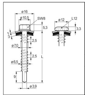
Fastener: Stainless steel A2 or A4 - EN ISO 3506 Washer: Stainless steel A2 or A4 - EN ISO 3506
