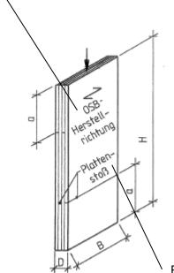
Compression load parallel to the direction of construction of the OSB slabs.
