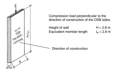
Direction of construction = direction of the grain of the surface layers
