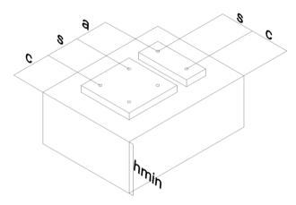
Fixing points with a spacing a  $\leq$  s<sub>cr,N</sub> are considered as a group with a maximum characteristic resistance N<sub>Rk,p</sub> acc. to Table 17 – Table 27. For a spacing a > s<sub>cr,N</sub> the anchors are considered as single anchors, each with a characteristic resistance N<sub>Rk,p</sub> acc. to Table 17 – Table 27.
