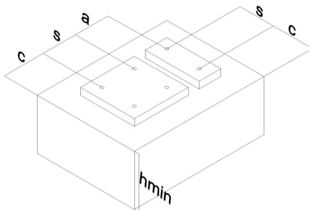
Fixing points with a spacing  $a \leq s_{cr,N}$  are considered as a group with a maximum characteristic resistance  $N_{Rk,p}$  acc. to Table 17 – Table 27. For a spacing  $a > s_{cr,N}$  the anchors are considered as single anchors, each with a characteristic resistance  $N_{Rk,p}$  acc. to Table 17 – Table 27.
