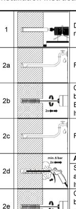
Drill with diamond drill a hole into the base material to the size and embedment depth required by the selected anchor (Table B1 or Table B2).
