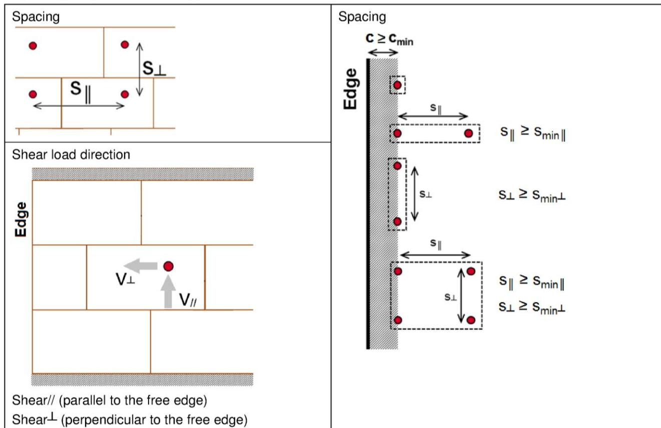
The characteristic values of resistance of an anchor group are calculated by using the group-factors  $\alpha_g$  according to Annexes C3 to C30:
