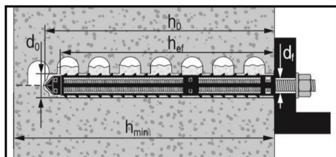
**Figure A3:** Solid brick with threaded rod, HIT-V-... (see Table B8)
