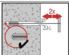
Brush 2 times with the specified steel brush (tables B5 to B10) by inserting the steel brush Hilti HIT-RB to the back of the hole (if needed with extension) in a twisting motion and removing it.
