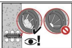
Control amount of injected mortar. Adhesive has to protrude into the lid.
