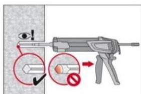
Inject the adhesive starting at the back of the hole, slowly withdrawing the mixer with each trigger pull.
