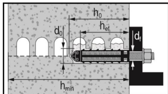
**Figure A2:** Hollow and solid brick with threaded rod, HIT-V-... and two sieve sleeves HIT-SC for deeper embedment depth (see Table B6)
