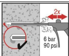
Blow again with Hilti hand pump or compressed air 2 times until return air stream is free of noticeable dust.
