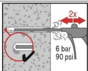
Blow 2 times from the back of the hole (if needed with nozzle extension) over the hole length with Hilti hand pump (drill hole diameter  $d_0 \leq 18$  mm and drill hole depth up to  $h_0 = 100$  mm) or oil-free compressed air (min. 6 bar at 6 m<sup>3</sup>/h; drill hole depth up to  $h_0 = 300$  mm) until return air stream is free of noticeable dust.
