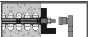
After required curing time  $t_{cure}$  (see Table B11 and Table B12) the anchor can be loaded.
