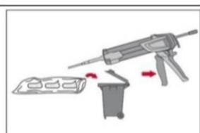
Discard initial adhesive. The foil pack opens automatically as dispensing is initiated. Depending on the size of the foil pack an initial amount of adhesive has to be discarded. Discarded quantities are
