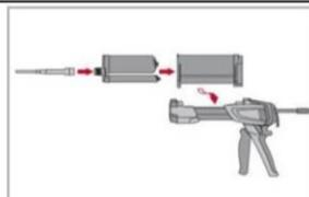
Tightly attach new Hilti mixing nozzle HIT-RE-M to foil pack manifold (snug fit). Do not modify the mixing nozzle.
