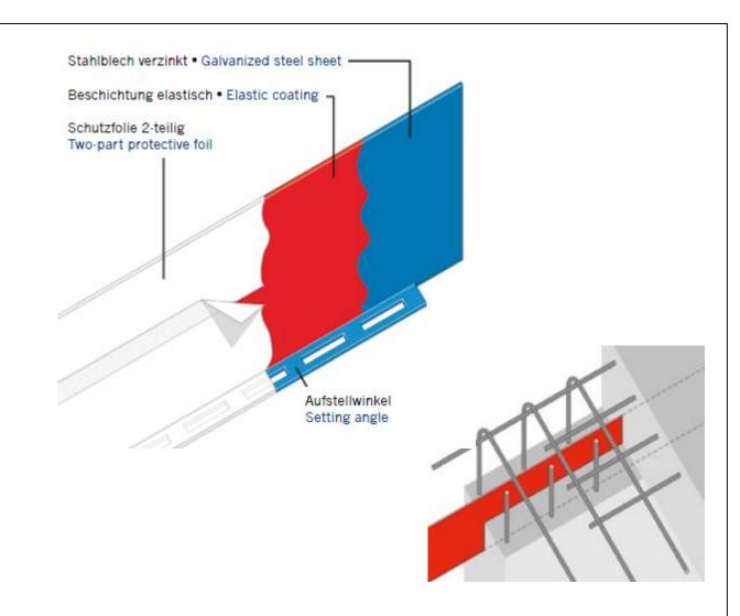
WP sealing sheet BK, h = 150 mm or 80 mm WFP sealing sheet BGL 150 (without setting angle), h = 150 mm
