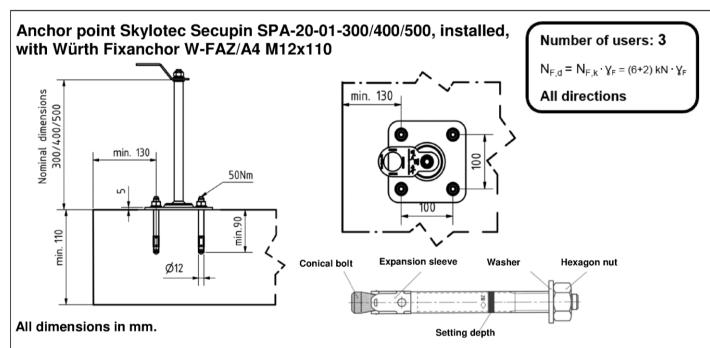
Installation instructions for anchor point Skylotec Secupin SPA-20-01-300/400/500 with Würth Fixanchor W-FAZ/A4 M12x110
