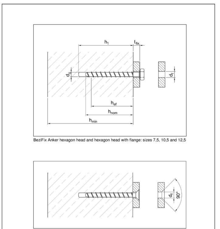
BeziFix Anker countersunk head: size 7,5
