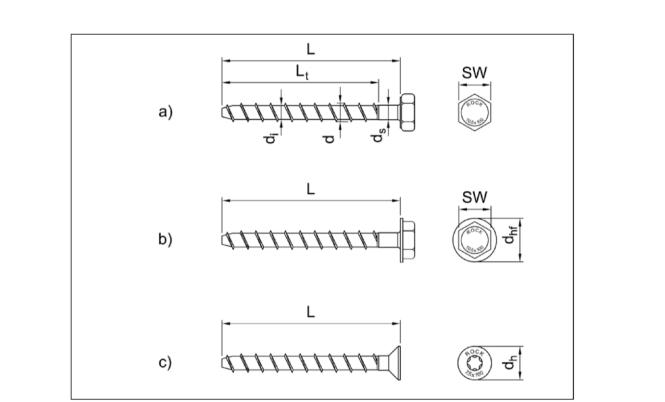
**Screw types:** a) BeziFix Anker hexagon head 7,5, 10,5 and 12,5. b) BeziFix Anker hexagon head with flange 7,5, 10,5 and 12,5. c) BeziFix Anker countersunk head 7,5. Head marking: "Rock" and size x screw length.
