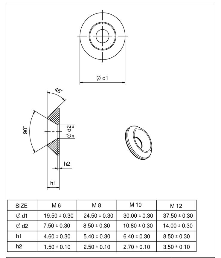
BeFIX, BeFIX D & BeFIX V screws
