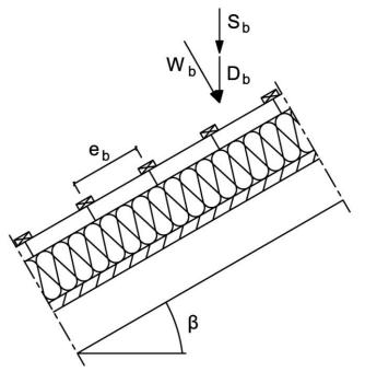
Figure A.4.2 Point loads  $F_{\rm b}$  perpendicular to the battens
