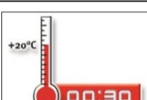
10. Allow the adhesive to cure to the specified time prior to applying any load or torque. Do not move or load the anchor until it is fully cured (attend Table B5).
