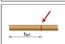
4. Prior to inserting the anchor rod into the filled bore hole, the position of the embedment depth shall be marked on the anchor rods.
