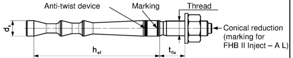
**Marking:** work symbol, size of anchor, setting depth. e.g.:
