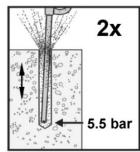
Blow 2 times with oil-free compressed air (min. 5.5 bar) and verify that the threaded rod and rebar can achieve the required embedment depth.
