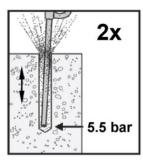
Blow dust from hole 2 times with oil-free compressed air (min. 5.5 bar) starting from the bottom of the hole.
