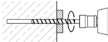
3. Installing the concrete screw through the fixture using an impact screw driver
