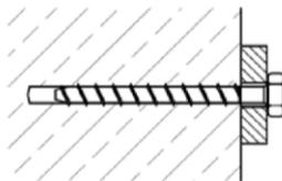
4. Fixture is fully pressed onto the surface of the concrete member without intermediate layer
