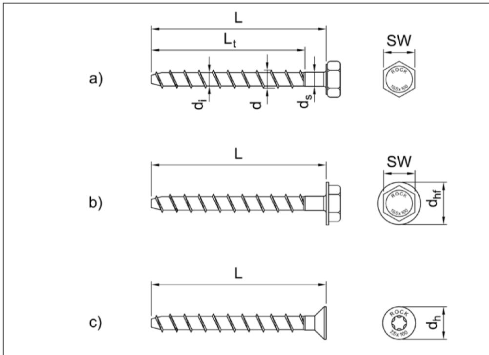
**Screw types:** a) BeziFix Anker hexagon head 7,5, 10,5 and 12,5.
