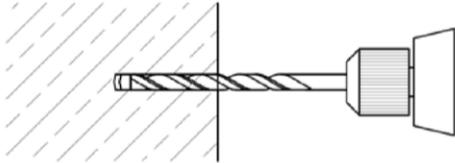
1. Drilling the hole by hammer drilling
