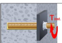
11. After full curing, the add-on part can be installed with up to the max. torque (Table B1 or B3) by using a calibrated torque wrench.
