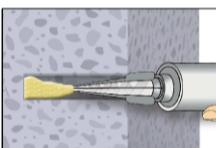
6. Starting from the bottom or back of the cleaned anchor hole, fill the hole up to approximately two-thirds with adhesive. Slowly withdraw the static mixing nozzle as the hole fills to avoid creating air pockets. For embedment larger than 190 mm an extension nozzle shall be used. Observe the gel-/ working times given in Table B5.
