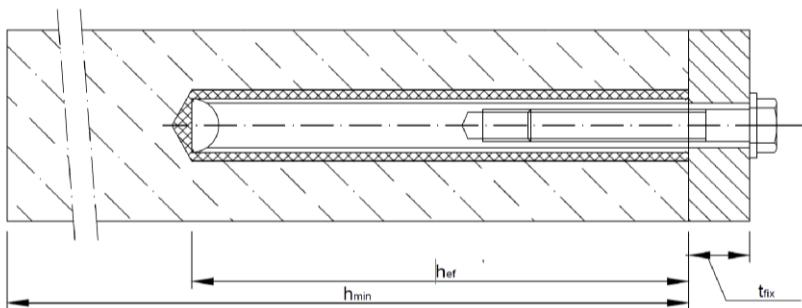
$t_{\text{fix}}$  = thickness of fixture
