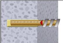
8. Push the threaded rod or reinforcing bar into the anchor hole while turning slightly to ensure positive distribution of the adhesive until the embedment depth is reached.
