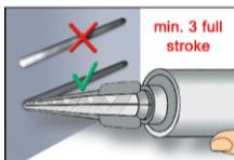
5. Prior to dispensing into the anchor hole, squeeze out separately a minimum of three full strokes and discard non-uniformly mixed adhesive components until the mortar shows a consistent grey colour.
