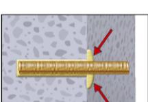
9. Be sure that the anchor is fully seated at the bottom of the hole and that excess mortar is visible at the top of the hole. If these requirements are not maintained, the application has to be renewed. For overhead application the anchor rod shall be fixed (e.g. wedges).
