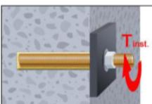
11. After full curing, the add-on part can be installed with up to the max. torque (Table B1 or B3) by using a calibrated torque wrench.
