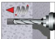
1. Drill with hammer drill a hole into the base material to the size and embedment depth required by the selected anchor (Table B1, B2, or B3). In case of aborted drill hole: the drill hole shall be filled with mortar
