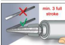
5. Prior to dispensing into the anchor hole, squeeze out separately a minimum of three full strokes and discard non-uniformly mixed adhesive components until the mortar shows a consistent grey colour.
