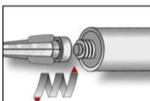
3. Attach the supplied static-mixing nozzle to the cartridge and load the cartridge into the correct dispensing tool.
