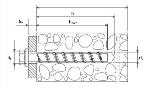
$\begin{array}{lll} d_0 & = & \text{nominal drill bit diameter} \\ h_{\text{nom}} & = & \text{nominal anchorage depth} \\ h_1 & = & \text{depth of the drill hole} \end{array}$
