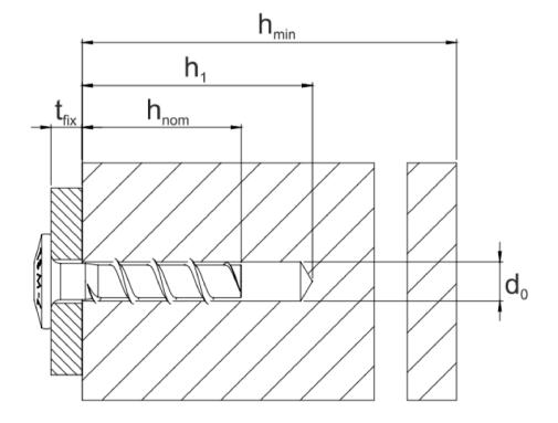
$\begin{array}{lll} h_{nom} & = & nominal \ anchorage \ depth \\ h_1 & = & depth \ of \ the \ drill \ hole \\ h_{min} & = & thickness \ of \ member \\ t_{fix} & = & thickness \ of \ fixture \end{array}$
