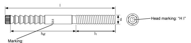
Embossing: "M..xh $_{nom}/I_1$  G8.8" hot dip galvanized steel (HIT CS-F) (e.g. M16x125/85 G8.8)
