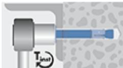
Tightening with torque wrench and predetermined value of  $T_{inst}$
