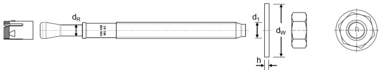
Figure A1: Hilti metal expansion anchor HSB
