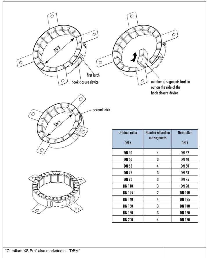
Design of the pipe collar in the size DN 32 to DN 200
