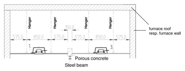
2 x 12.5 mm gypsum plaster fire protection boards
