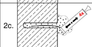
2c. Starting from the bottom or back of the bore hole blow out the hole again a minimum of **four** times.
