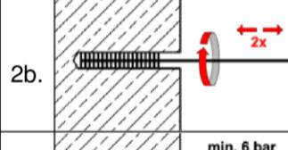
2b. Check brush diameter (Table B4). Brush the hole with an appropriate sized wire brush  $\geq d_{b,min}$  (Table B4) a minimum of **two** times. If the bore hole ground is not reached with the brush, a brush extension must be used.
