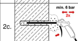
2c. Starting from the bottom or back of the bore hole, blow out the hole with compressed air (min. 6 bar) again a minimum of **two** times until return air stream is free of noticeable dust. If the bore hole ground is not reached, an extension must be used.
