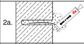
2a. Starting from the bottom or back of the bore hole, blow out the hole with the blow-out pump a minimum of **four** times.
