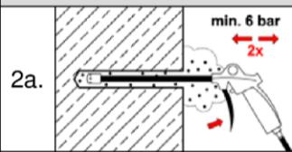
2a. Starting from the bottom or back of the bore hole, blow out the hole with compressed air (min. 6 bar) a minimum of **two** times until return air stream is free of noticeable dust. If the bore hole ground is not reached, an extension must be used.
