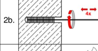
2b. Check brush diameter (Table B4). Brush the hole with an appropriate sized wire brush  $\geq d_{b,min}$  (Table B4) a minimum of **four** times. If the bore hole ground is not reached with the brush, a brush extension must be used.
