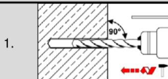
1. Drill with hammer drill or compressed air drill or vacuum drill a hole into the base material to the size required by the selected anchor (Table B1, B2 or Table B3). In case of aborted drill hole, the drill hole shall be filled with mortar.
