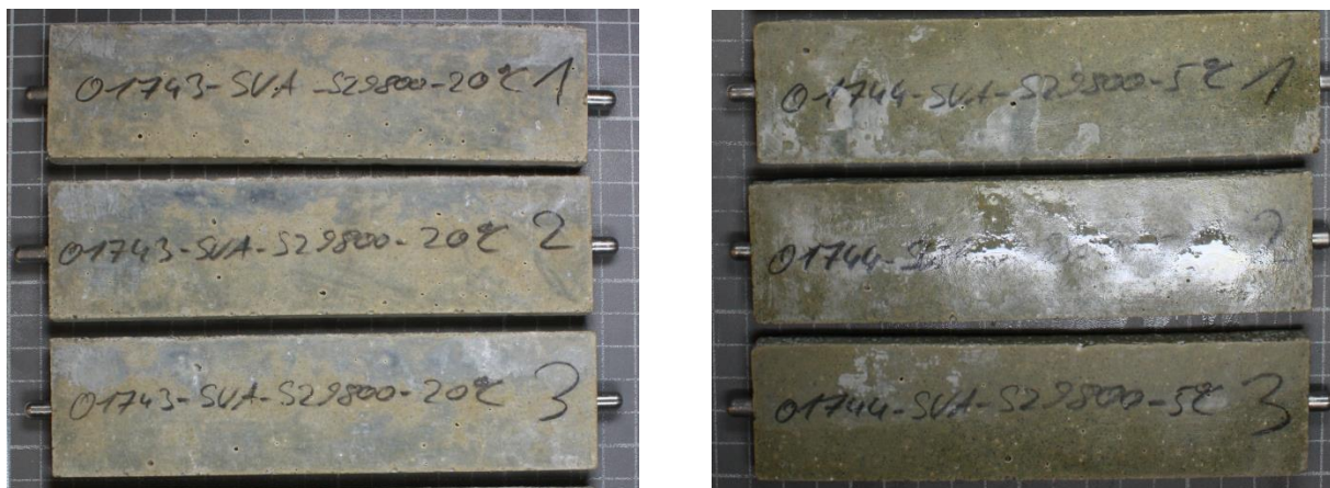
Figure 7: Specimens with CEM III/B 42,5 N-LH/SR after 180 days; Storage: in Na 2 O 4 -Solution at 20 °C (on the left) and at 5 °C (on the right)
