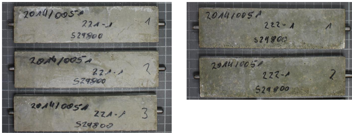
Figure 3: Specimens with CEM III/B 42,5 N-LH/SR after 180 days; Storage: in \text{Na}_2\text{O}_4 -Solution at 20 °C (on the left) and at 5 °C (on the right)
