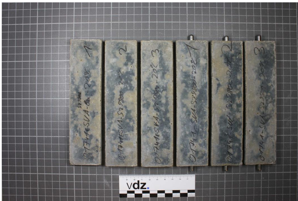
Figure 5: Specimens with CEM III/A 52,5 N-SR/LA "Duisburg" with blast furnace slag 2 (S2) after 180 days; Storage: 20 °C in Na 2 O 4 -Solution
