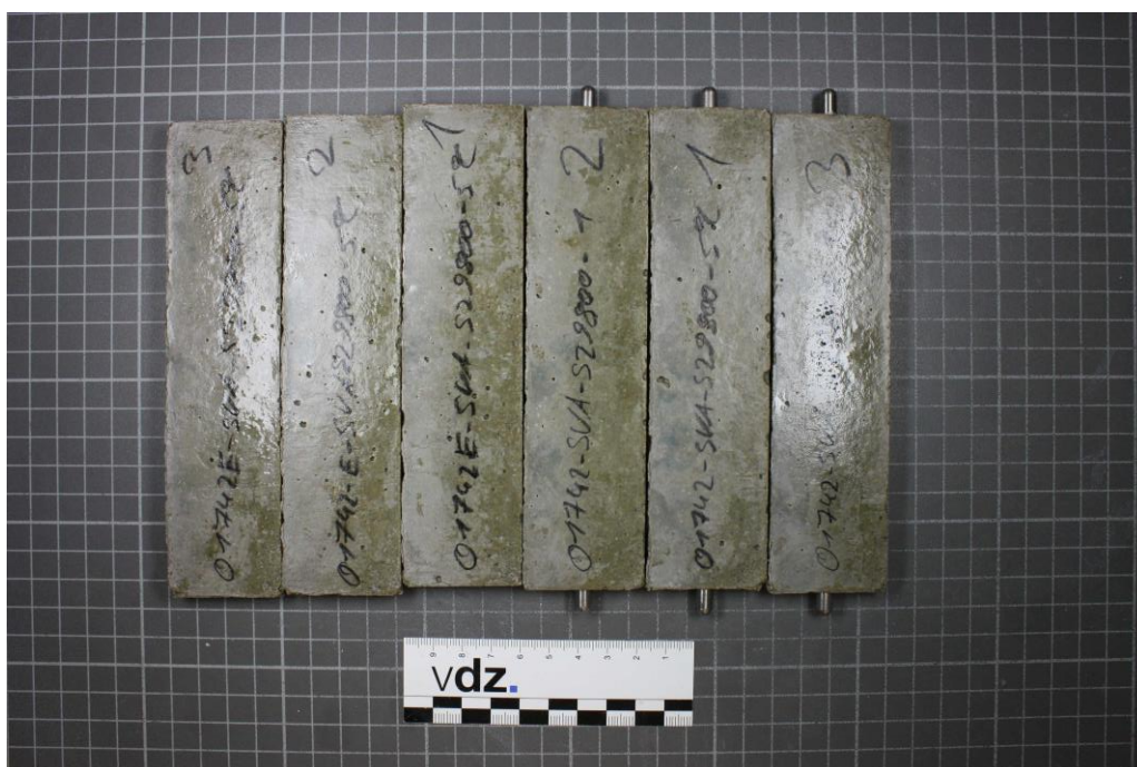
Figure 6: Specimens with CEM III/A 52,5 N-SR/LA "Duisburg" with blast furnace slag 2 (S2) after 180 days; Storage: 5 °C in Na 2 O 4 -Solution
