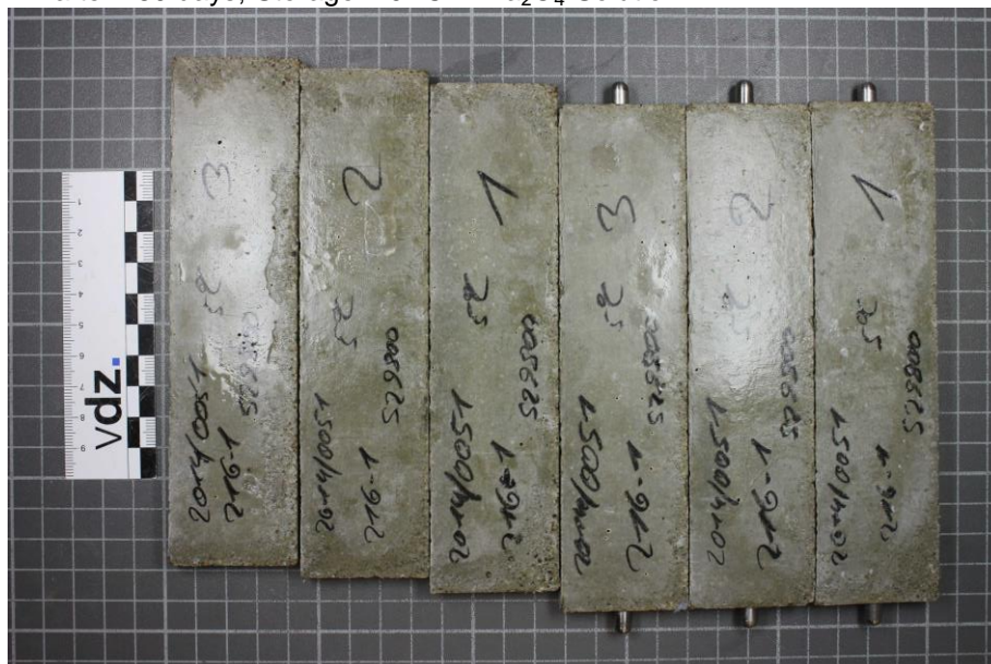
Figure 2: Specimens with CEM III/A 52,5 N-SR/LA "Duisburg" with blast furnace slag 1 (S1) after 180 days; Storage: 5 °C in Na_2O_4 -Solution
