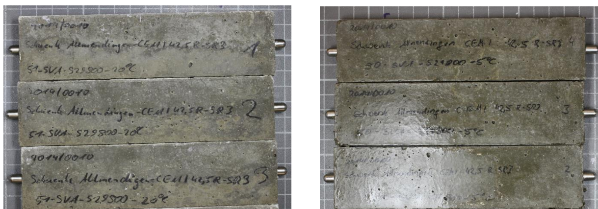
Figure 8: Specimens with CEM I 42,5 R-SR3 after 180 days; Storage: in Na 2 O 4 -Solution at 20 °C (on the left) and at 5 °C (on the right)
