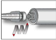
3. Attach the supplied static-mixing nozzle to the cartridge and load the cartridge into the correct dispensing tool.
