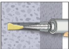
6. Starting from the bottom or back of the cleaned anchor hole, fill the hole up to approximately two-thirds with adhesive. Slowly withdraw the static mixing nozzle as the hole fills to avoid creating air pockets. For embedment larger than 190 mm an extension nozzle shall be used. Observe the gel-/ working times given in Table B5.
