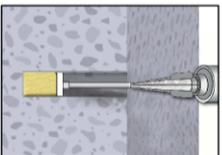
7. Piston Plugs and mixer nozzle extensions shall be used according to Table B4 for the following applications:
