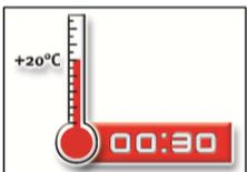
10. Allow the adhesive to cure to the specified time prior to applying any load or torque. Do not move or load the anchor until it is fully cured (attend Table B5).
