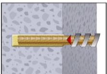
8. Push the threaded rod or reinforcing bar into the anchor hole while turning slightly to ensure positive distribution of the adhesive until the embedment depth is reached.
