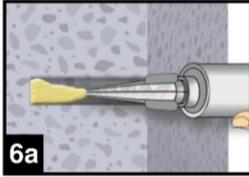
6. Starting from the bottom or back of the cleaned anchor hole fill the hole up to approximately two-thirds with adhesive. Slowly withdraw the static mixing nozzle as the hole fills to avoid creating air pockets. For embedment larger than 190 mm an extension nozzle shall be used.
