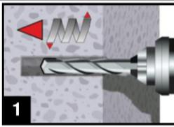
1. Drill a hole into the base material to the size and embedment depth required by the selected reinforcing bar with carbide hammer drill (HD) or a compressed air drill (CD). In case of aborted drill hole: the drill hole shall be filled with mortar.
