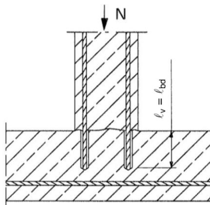
**Figure A5:** Anchoring of reinforcement to cover the line of acting tensile force
