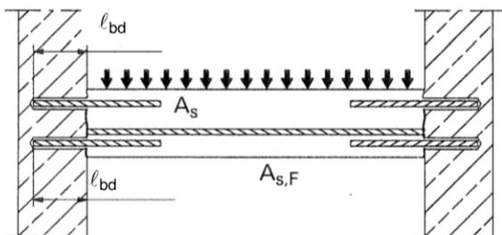
**Figure A4:** Rebar connection for components stressed primarily in compression. The rebars are stressed in compression
