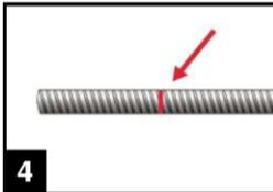
4. Prior to inserting the reinforcing bar into the filled bore hole, the position of the embedment depth shall be marked (e.g. with tape) on the reinforcing bar and insert bar in empty hole to verify hole and depth  $l_v$ .
