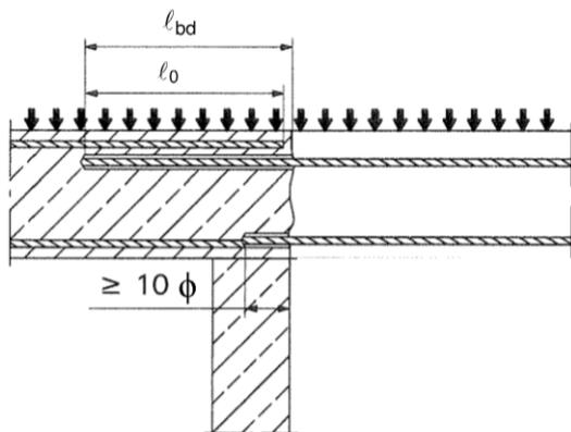
**Figure A2:** Overlapping joint at a foundation of a wall or column where the rebars are stressed in tension
