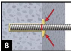
8. Be sure that the bar is inserted in the bore hole until the embedment mark is at the concrete surface and that excess mortar is visible at the top of the hole. If these requirements are not maintained, the application has to be renewed. For overhead installation fix embedded part (e.g. wedges).
