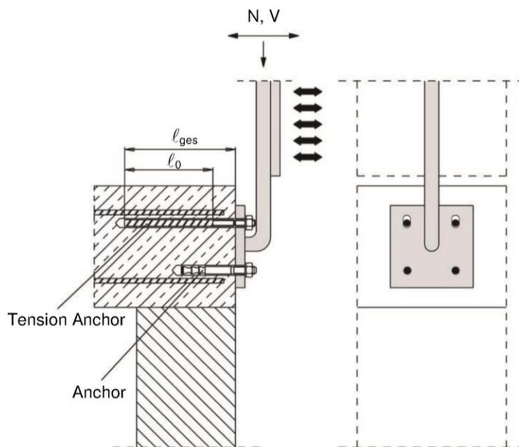
**Figure A8:** Overlap joint for the anchorage to cantilever members
