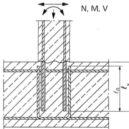
**Figure A3:** End anchoring of slabs or beams (e.g. designed as simply supported)
