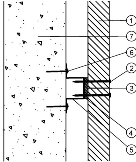
detail fastening of cladding made of fire protective boards
