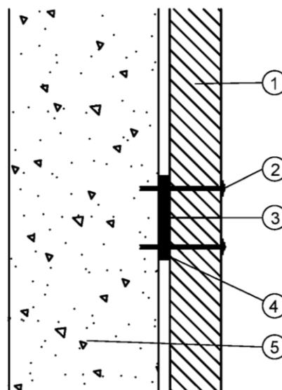
detail fastening of cladding made of fire protective boards
