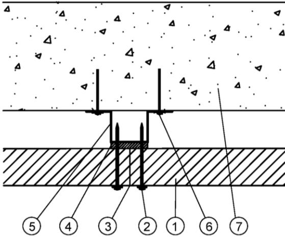
section wall with cladding made of fire protective boards
