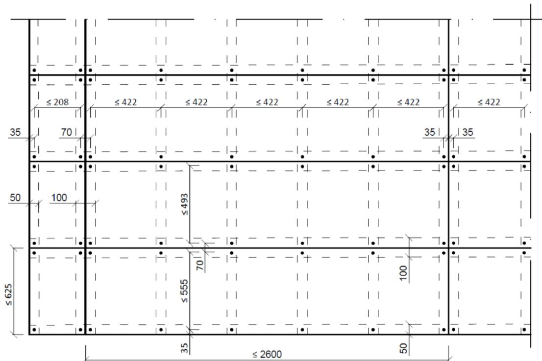
cladding with 30mm thick fire protective boards
