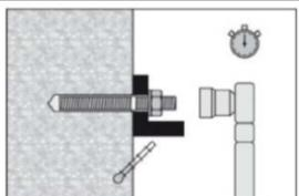
Loading the anchor: After required curing time  $t_{cure}$  (see Table B3) the anchor can be loaded.
