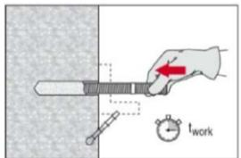
Before use, verify that the element is dry and free of oil and other contaminants. Mark and set element to the required embedment depth until working time  $t_{work}$  has elapsed. The working time  $t_{work}$  is given in Table B3
