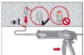
Overhead installation and/or installation with embedment depth  $h_{ef} > 250\text{mm}$ . For overhead installation the injection is only possible with the aid of extensions and piston plugs. Assemble HIT-RE-M mixer, extension(s) and appropriately sized piston plug HIT-SZ (see Table B4). Insert piston plug to back of the hole and inject adhesive. During injection the piston plug will be naturally extruded out of the drill hole by the adhesive pressure
