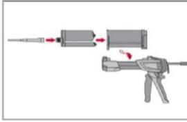
Tightly attach new Hilti mixing nozzle HIT-RE-M to foil pack manifold (snug fit). Do not modify the mixing nozzle.
