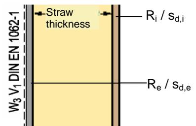
c) Roof structures with ventilated roofing
