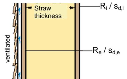
b) Plastered exterior wall structures with no weather protection
