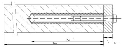
$t_{fix}$  = thickness of fixture
