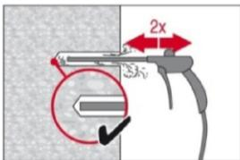
Blow 2 times from the back of the hole (if needed with nozzle extension) over the entire hole length with oil-free compressed air (min. 6 bar at 6 m<sup>3</sup>/h) until return air stream is free of noticeable dust.
