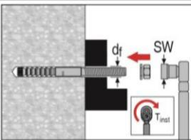
After required curing time  $t_{cure}$  (see Table B2) remove excess mortar. Assemble the washer and the first nut and apply the installation torque. The required installation torque  $T_{inst}$  is given in Table B1.
