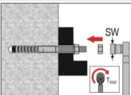
Assemble the second nut and apply the installation torque. The required installation torque  $T_{inst}$  is given in Table B1. After torquing the anchor can be loaded.
