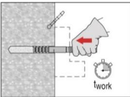
Before use, verify that the anchor rod is dry and free of oil and other contaminants. Set the anchor rod to the required embedment depth before working time  $t_{work}$  has elapsed. The working time  $t_{work}$  is given in Table B2.
