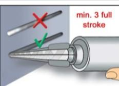
2. Initial adhesive is not suitable for fixing the anchor. Prior to dispensing into the anchor hole, squeeze out separately a minimum of three full strokes, for foil tube cartridges six full strokes and discard non-uniformly mixed adhesive components until the mortar shows a consistent grey colour.
