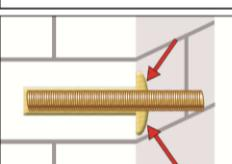
7. Be sure that the anular gap is fully filled with mortar. If no excess mortar is visible at the top of the hole, the application has to be renewed.
