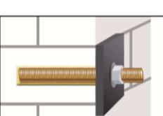
9. After full curing, the fixture can be installed with up to the max. installation torque (see Annex B4) by using a calibrated torque wrench.
