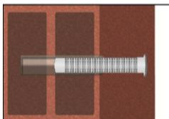
5. Insert the perforated sleeve flush with the surface of the masonry or plaster. Only use sleeves that have the right length. Never cut the sleeve.
