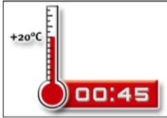
8. Allow the adhesive to cure to the specified curing time prior to applying any load or torque. Do not move or load the anchor until it is fully cured (attend Table B4 and B5).
