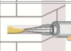
5. Starting from the bottom or back of the cleaned anchor hole, fill the hole up to min two-thirds with adhesive. Slowly withdraw the static mixing nozzle will avoid creating air pockets. Observe the gel-/ working times given in Table B4 and B5.
