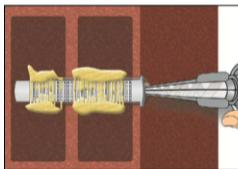
6. Starting from the bottom or back fill the sleeve with adhesive. For embedment depth equal to or larger than 130 mm an extension nozzle shall be used. For quantity of mortar attend cartridges label installation instructions.
