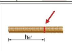
6. The position of the embedment depth shall be marked on the threaded rod. Push the threaded rod into the anchor hole while turning slightly to ensure positive distribution of the adhesive until the embedment depth is reached. The anchor shall be free of dirt, grease, oil or other foreign material.
