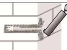
4. Blow out from the bottom of the bore hole two times. Attach the appropriate sized brush ( $> d_{b,min}$  Table B2 or B3) to a drilling machine or a battery screwdriver, brush the hole clean two times, and finally blow out the hole again two times.
