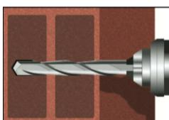
3. Holes to be drilled perpendicular to the surface of the base material by using a hard-metal tipped hammer drill bit. Drill a hole, with drill method according to Annex C4 – C45, into the base material, with nominal drill hole diameter and bore hole depth according to the size and embedment depth required by the selected anchor.
