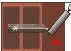
4. Blow out from the bottom of the bore hole two times. Attach the appropriate sized brush ( $> d_{b,min}$  Table B3) to a drilling machine or a battery screwdriver, brush the hole clean two times, and finally blow out the hole again two times.
