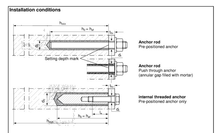
Injection system PfT bonded mortar
