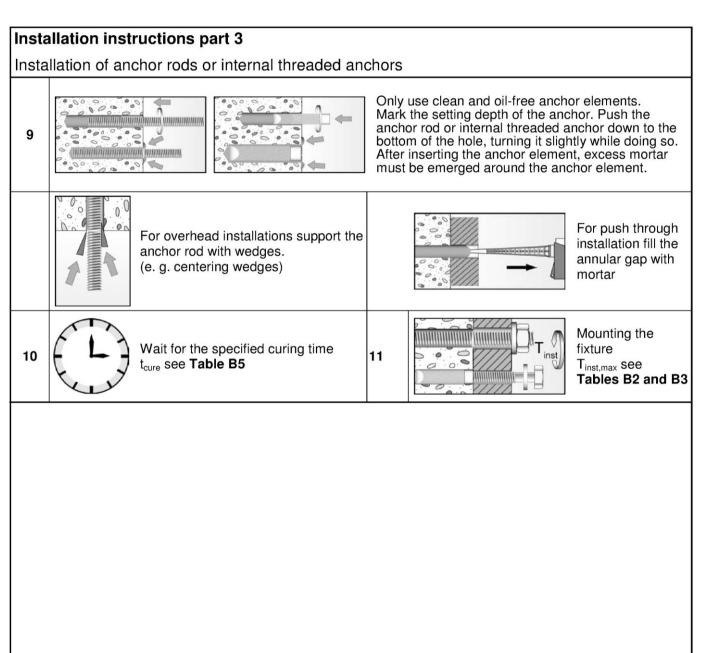
Injection system PfT bonded mortar
