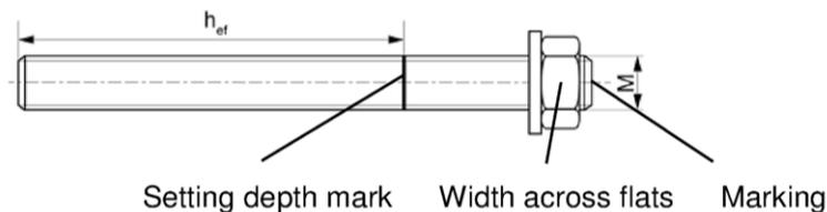
**Anchor rod with roof cutting**
