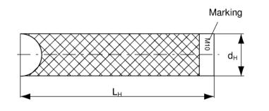
Marking: Anchor size e. g.: M10 Stainless steel additional A4
