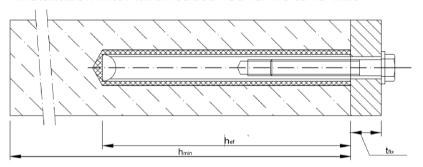
$t_{fix}$  = thickness of fixture
