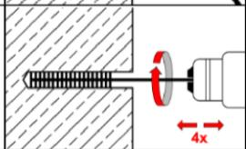
Attach the brush to a drilling machine or a battery screwdriver. Brush the hole with an appropriate sized wire brush  $> d_{b,min}$  (Table B4) **four** times.
