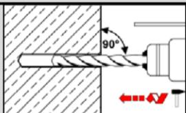
Drill the borehole by applying the drilling method acc. to Annex B1, the drill bit diameter (Table B4) and the selected borehole depth.
