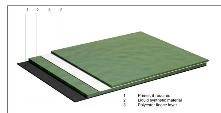
Applicable to the roof waterproofing "Triflex ProTect":
