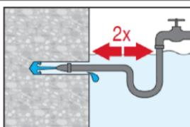
Flush another 2 times by inserting a water hose (water-line pressure) to the back of the hole until water runs clear.
