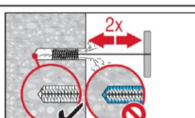
Brush 2 times with the specified brush size (brush  $\varnothing \geq$  drill hole  $\varnothing$ , see Table B7) by inserting the steel brush Hilti HIT-RB to the back of the hole (if needed with extension) in a twisting motion and removing it.
