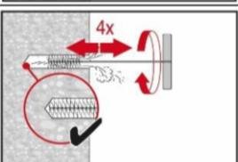
Brush 4 times with the specified brush (see Table B7) by inserting the steel brush Hilti HIT-RB to the back of the hole (if needed with extension) in a twisting motion and removing it.
