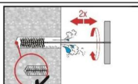
Brush 2 times with the specified brush (see Table B7) by inserting the steel brush Hilti HIT-RB to the back of the hole (if needed with extension) in a twisting motion and removing it.
