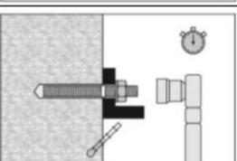
Loading the anchor: After required curing time  $t_{cure}$  (see Table B6) the anchor can be loaded.
