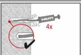
The Hilti hand pump may be used for blowing out drill holes up to diameters  $d_0 \leq 18 \text{ mm}$  and embedment depths up to  $h_{ef} \leq 10 \cdot d$ .
