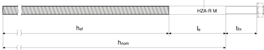
**Table B5: Installation parameters of reinforcing bar (rebar)**
