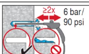
Blow 2 times from the back of the hole (if needed with nozzle extension) over the whole length with oil-free compressed air (min. 6 bar at 6 m³/h) until return air stream is free of noticeable dust and water.
