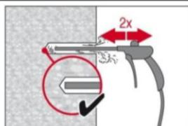
Blow 2 times from the back of the hole (if needed with nozzle extension) over the whole length with oil-free compressed air (min. 6 bar at 6 m<sup>3</sup>/h) until return air stream is free of noticeable dust.
