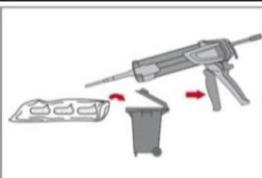
The foil pack opens automatically as dispensing is initiated. Depending on the size of the foil pack an initial amount of adhesive has to be discarded.
