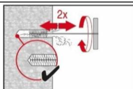
Brush 2 times with the specified brush (see Table B7) by inserting the steel brush Hilti HIT-RB to the back of the hole (if needed with extension) in a twisting motion and removing it.
