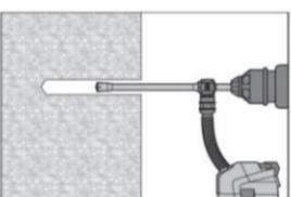
Drill hole to the required embedment depth with an appropriately sized Hilti TE-CD or TE-YD hollow drill bit attached to Hilti vacuum cleaner VC 20/40 (-Y) (suction volume  $\geq 57 \text{ l/s}$ ) with automatic cleaning of the filter activated. This drilling system removes the dust and cleans the drill hole during drilling when used in accordance with the user's manual.
