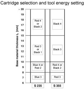
Note for S 275: Start with recommendation for S 355. In case of too much energy: Reduction of tool energy setting or change of cartridge colour till correct stand-offs  $h_{\text{NVS}}$  are achieved.
