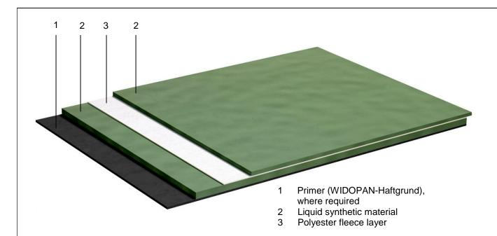
Applicable to the roof waterproofing "WIDOPAN-FD" / "WIDOPAN-Plus":
