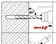
Drill hole perpendicular to concrete surface, positioning of the drill holes without damaging the reinforcement.
