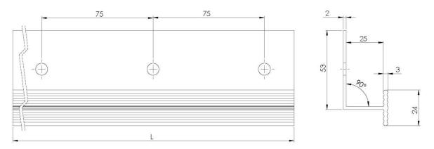
Vertical connection profile – "SCHWEPA Verbindungsleiste PVC" (dimensions in millimetres)
