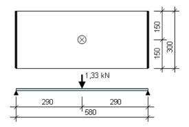
$\sigma_{FE}$  = maximum main tensile stress [N/mm<sup>2</sup>]
