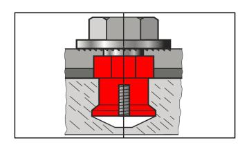
b) Installed anchor
