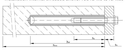
$t_{fix}$  = thickness of fixture
