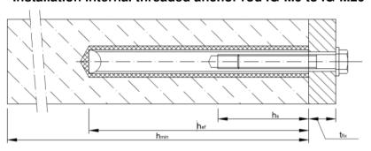
$t_{fix}$  = thickness of fixture
