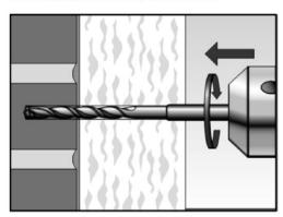
1. Drill the bore hole by the parameters acc. to Table B2.1 and the corresponding drilling method acc. to Annex C 1.
