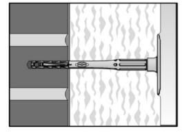
4. Correctly installed anchor.
