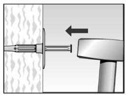
3. Set anchor by hammer blows. The bottom side of the plate must be flush with the ETICS.
