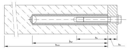
$t_{fix}$  = thickness of fixture
