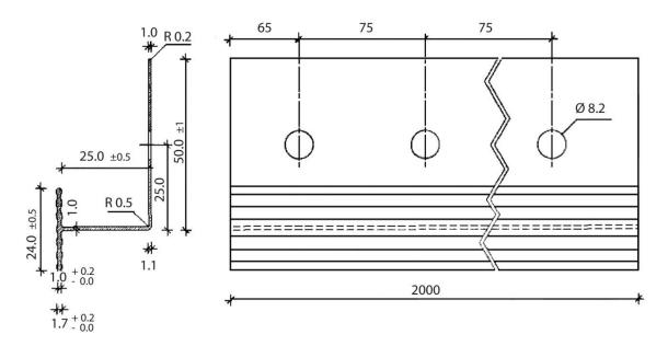
Vertical connection profile - "SCHWEPS Verbindungsleiste Alu" (dimensions in millimetres)
