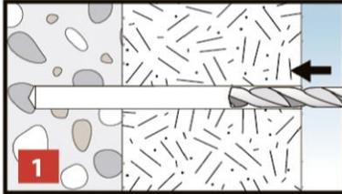
Create a hole considering the drill method according Annex C 1
