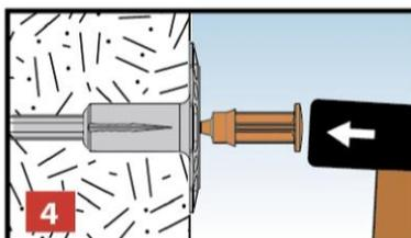
Hammer in the nail with a matching hammer
