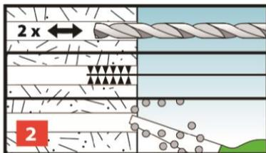
Holes to be cleaned of drilling dust.
